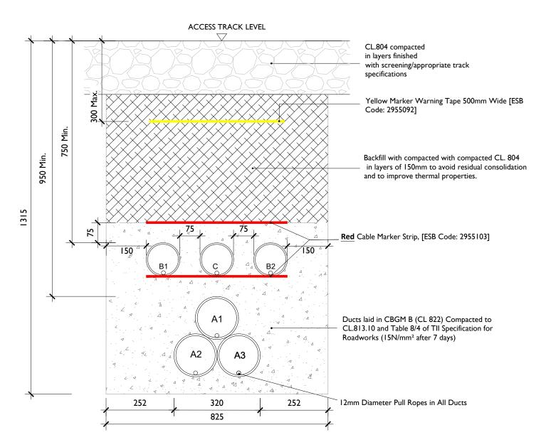
A = 160mm: Outer Diameter HDPE ESB Approved Duct, SDR= 21.0 (Power) [ESB Code: 9317560]
